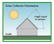
Today, most solar water heating collectors are mounted flat on the roof. This is more aesthetically pleasing than rack-mounted collectors, which stick up from the roof at odd angles. Thus, most collectors have the same tilt as the roof.
