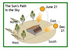
Solar hot water collectors should be oriented geographically to maximize the amount of daily and seasonal solar energy that they receive. In general, the optimum orientation for a solar collector in the northern hemisphere is true south. However, recent studies have shown that, depending on your location and collector tilt, your collector can face up to 90° east or west of true south without significantly decreasing its performance.
